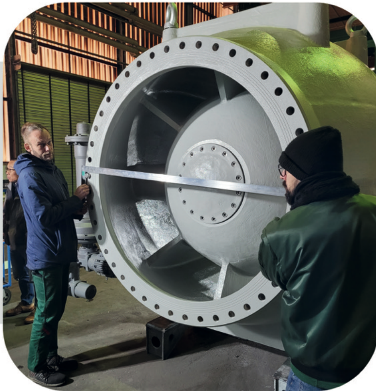
New plunger valve being measured for mounting bolt locations prior to shipment
